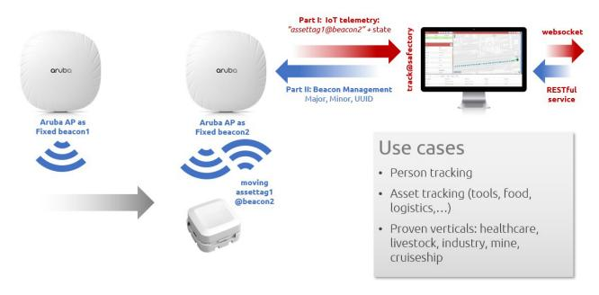
To set up Aruba access points to be used with safectory products (asset tags, beacons, mobile SDK, Track backend), use the following manual.
